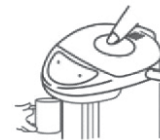
Figure of dispensing water by manual pumping
