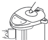
Figure of dispensing water by manual pumping
